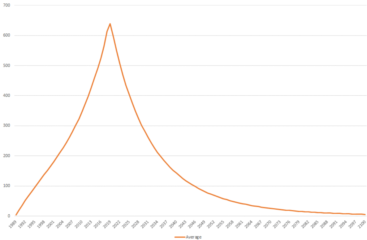
Figure 3 Wood 2018 bulk gas generation estimate (m 3 /hr)
